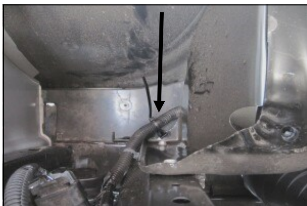
7. Secure the wiring harness to the inner fender as shown using the Edge Clip Cable Tie (#13).
