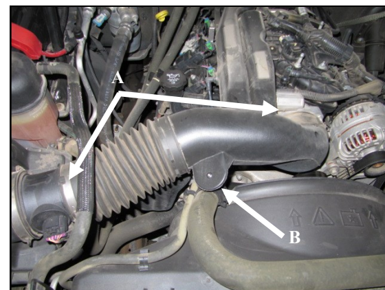
3.A.) Loosen the clamps securing the factory intake tube to the throttlebody and the Mass Air Flow Meter, or MAF.
