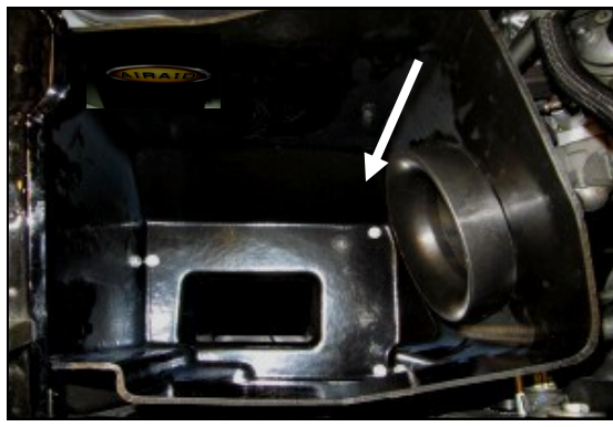
11. Install the Airaid CAB into the vehicle replacing the factory airbox. Secure the CAB using the three of the factory 6mm bolts from step 8. Do not over tighten. Apply the Airaid decal inside the Airbox as shown.
