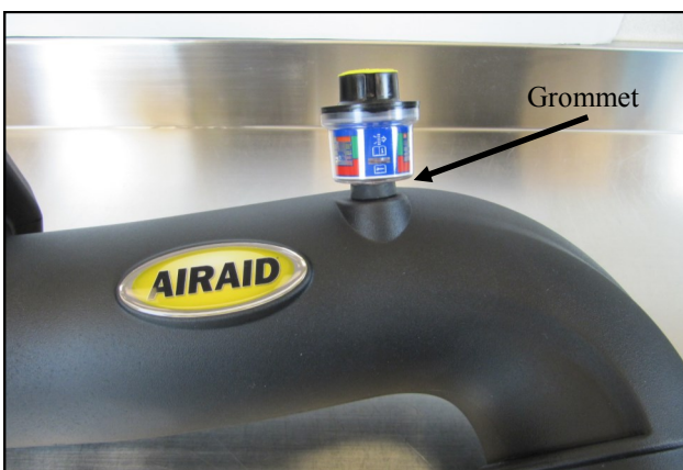
7. Install the 1/2" Grommet into the Airaid Intake Tube and transfer the OEM filter minder into it. Do not use the factory Grommet.
