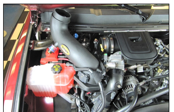
9. Slide the Airaid Intake Tube under the coolant hose and up the against the cowl as shown.
