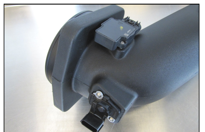
6. Transfer the Mass Air Flow sensors into the Airaid Intake Tube and secure them using two 8-32 x 1/2" Button Head Screws (#9) Do Not Use Factory Screws!
