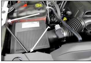
**6.** On 2015 Models: Remove the two 6mm bolts in the fender brace and set the bolts and brace to the side.
