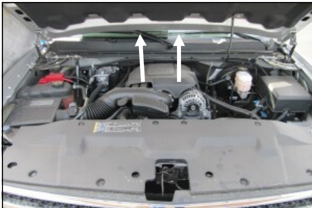
1. Disconnect the negative battery cable. Remove the engine cover by simply pulling up on it and sliding out from the vehicle.
