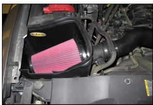
**14.** Install the Airaid Premium Filter (#1) onto the Filter Adapter, and tighten the hose clamp. Install the weather strip (#8) onto the Airaid Cold Air Box. (<u>Hint</u>: Start from one corner and work your way around for ease of install.)
