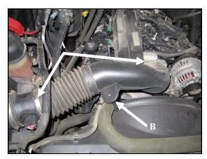
**3.A.)** Loosen the clamps securing the factory intake tube to the throttlebody and the Mass Air Flow Meter, or
