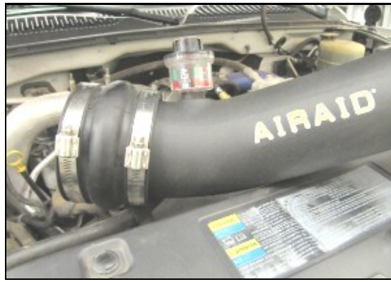
11. Install the urethane hump hose (#5) and two #72 hose clamps (#12) onto the large end of the Airaid Intake tube. (Note: Leave hose clamps loose until final assembly.)
