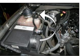
**3.** Remove the factory intake tube from the vehicle. Next, remove the **MAF** sensor and coupler from the factory airbox and set them out of the way without disconnecting the wiring harness.
