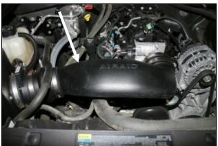
11. Install the small end of the intake tube into the hump hose first and then rotate it slightly to slide the other end into coupler on the throttlebody. Adjust for fit, and then tighten all four hose clamps.
