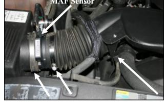
2. Loosen two hose clamps. One on each side of the Mass Air Flow (MAF) sensor.
