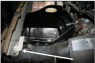
**8.** Install the **CAB** assembly into the vehicle where the factory airbox used to be using three 6mm hex bolts (#12) and three flat washers (#11) thru the bottom. Now reinstall the factory fender bolt thru the bracket and into the fender. Adjust the assembly for fit and tighten all bolts and nuts at this time. Apply the Airaid decal inside the Airbox as shown.
