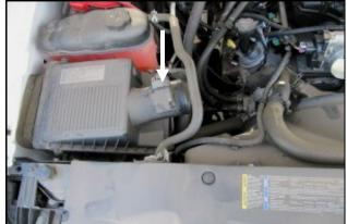
**5.** Disconnect the Mass Air Flow or MAF sensor and remove the factory airbox from the vehicle. The airbox is secured to the vehicle with grommets and simply lifts out.
