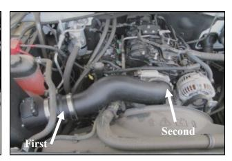
12. Install the Airaid Intake Tube assembly onto the Filter Adapter first, and then onto the throttlebody. Adjust for fit, and tighten all hose clamps. Reinstall the hose anchor into the Airaid Intake Tube.
