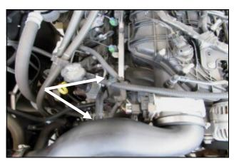
**13. A)** Install the 3/8" Breather Hose (#7) onto the Barbed Fitting and factory hard line.
