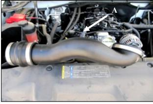
**11. A.)** Install the 3/8 NPT Fitting (#13) into the Airaid Intake Tube.
