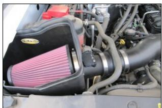
**14.** Install the Airaid Premium filter (#1) onto the Filter Adapter, and tighten the hose clamp. Install the Weather Strip (#8) onto the Airaid Cold Air Box. Reconnect the **M.A.F.** sensor. (*Hint: Start from one corner and work your way around for ease of install.*)
