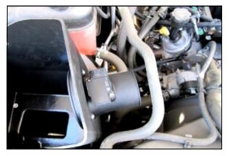
**10.** Transfer the Mass Air Flow sensor from the factory airbox into the Filter Adapter. Secure the sensor using the 8-32 Button Head Screws (#9).
