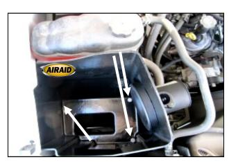
9. Install the CAB (#3) into the engine compartment and secure using three of the tray bolts from step 6. Apply the Airaid Foil Decal onto the Panel as shown.
