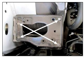
**6.** Remove the four tray bolts and the airbox mounting tray. Three of the bolts will be reused in step **9.**
