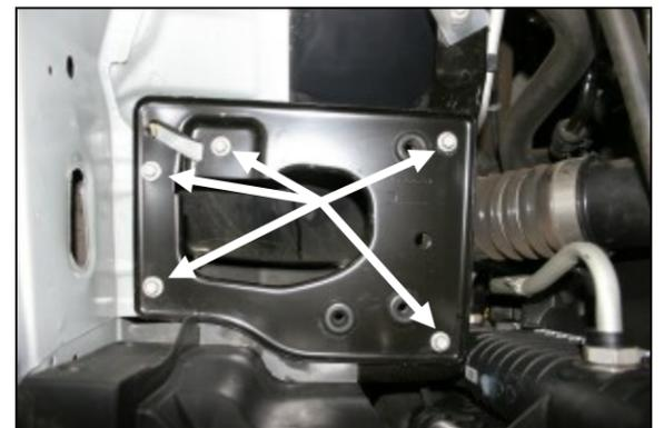
3. Using a 10mm socket, remove 5 bolts, and then remove the factory air filter mounting plate.
