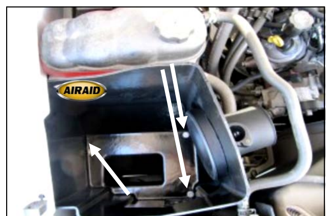
9. Install the CAB (#3) into the engine compartment and secure using three of the tray bolts from step 6. Apply the Airaid Foil Decal onto the Panel as shown.
