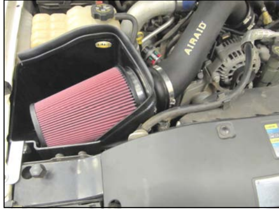
14. Install the Airaid Premium Filter (#1) onto the filter Adapter, and tighten the hose clamp. Install the Weather Strip (#7) onto the Airaid Cold Air Box. Reconnect the M.A.F. sensor wiring harness. ( Note: Start from one corner and work your way around to insure proper alignment of the weather strip. )
