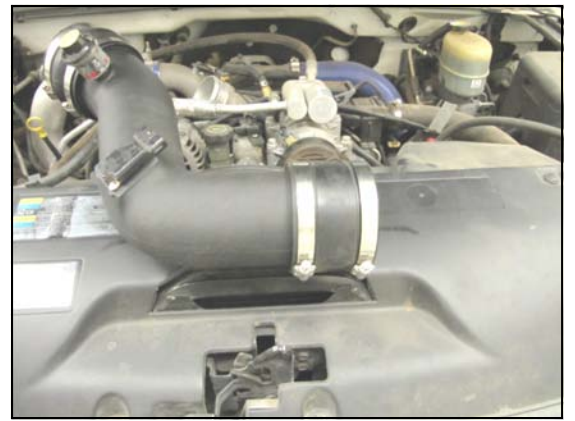
12. Install the urethane coupler (#6) and two #60 hose clamps (#11) onto the small end of the Airaid Intake tube. ( Note: Leave hose clamps loose until final assembly. )
