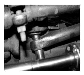
5. Install the New Fabtech adjustable Track Bar first at the lower pivot using thread lock and the factory nut. Tighten the nut to 183 ft-lbs. **SEE PHOTO BELOW**
