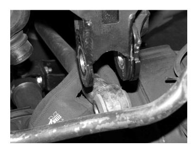
4. Locate the lower pivot ball joint assemble at the axle end of the track bar. Remove the nut attaching the bar to the ball joint in the axle. Retain the factory hardware and discard the factory Track Bar **SEE PHOTO BELOW.**
