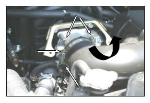
2. Using a 5/16" socket, loosen the hose clamp on the throttle body end of the factory air intake tube. Move the factory air intake tube up and out of the way of the throttle body. Using a 5mm allen wrench, remove the 4 bolts that hold the throttle body to the intake manifold.
