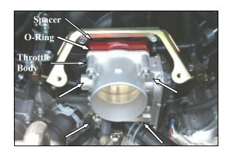
3. Install the O-Ring (#2) into the groove on the Poweraid Spacer (#1). Install the spacer between the intake manifold, and the throttle body with the O-Ring facing the throttle body. Insert four 6mm x 70mm Hex Bolts (#3), and 6mm Flat Washers (#4) through the throttle body, Poweraid Spacer, and into the intake manifold. Using a 10mm socket, tighten all 4 throttle body bolts evenly, to the manufacturer's specifications.
