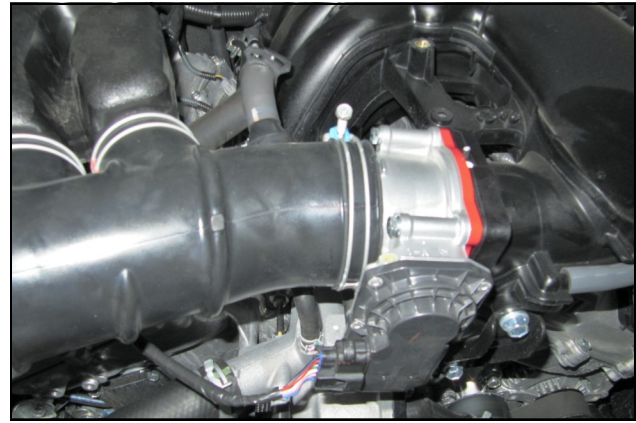
6. Reinstall the factory intake tube, tighten the two hose clamps, and reconnect the crankcase breather and Fuel pressure regulator lines. Reinstall the engine cover.
