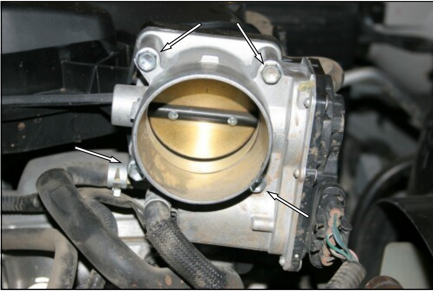
5. Using a 10mm socket, remove the 4 bolts that hold the throttlebody to the intake manifold.
