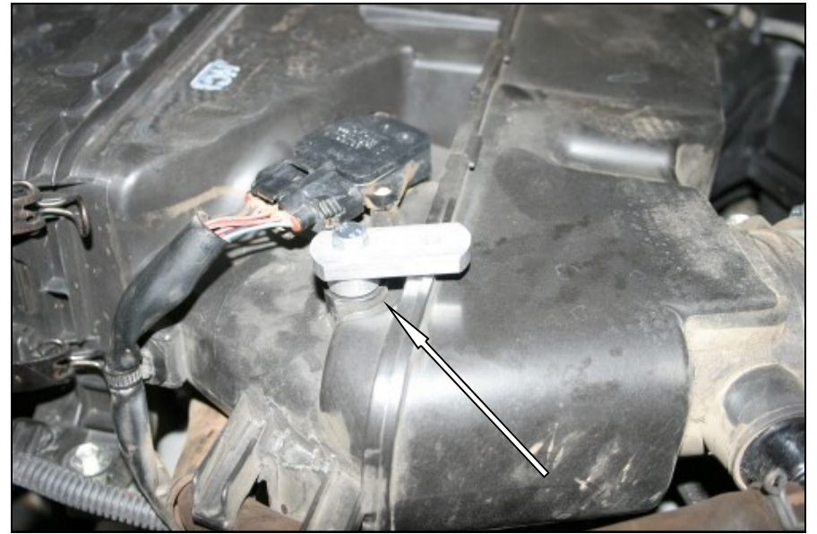
8. Reinstall the resonator/airbox assembly in the reverse order that you removed it using the factory bolts. Make sure to reconnect all breather and vacuum hoses, and the Mass Air sensor electrical connector. Install one 1" extension plate (#9) using the 5/16" thick round spacer (#10) and 6mm x 25mm bolt (#6), with flat washer (#4) in the threaded hole where the stud was removed on the resonator/airbox, with the extension plate facing the throttlebody as shown.
