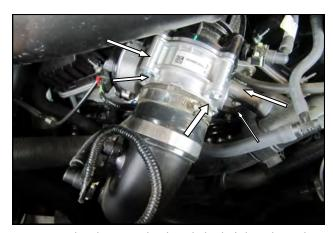
**2.** Loosen the clamp on the throttle body inlet tube and slide it away from the throttle body. Remove the four bolts that secure the throttle body to the intake manifold.
