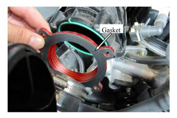
3. Pull the throttle body away from the intake manifold and Install the PowerAid and the supplied gasket. The logo is to be facing the throttle body and in the 12:00 o'clock position. the supplied gasket is to be on throttle body side. Align the bolt holes, and install the supplied bolts and washers. Tighten the bolts to the factory specifications in an "X" pattern. Before starting the engine, manually cycle the throttle plate to make sure there are no obstructions.
