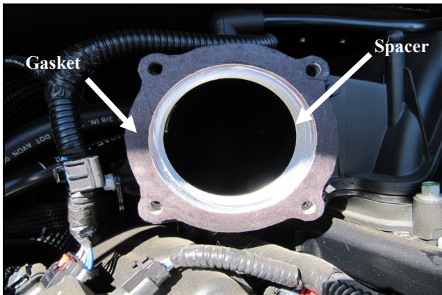
5. Insert the PowerAid spacer into the intake manifold. The gasket will go between the PowerAid and the throttlebody.
