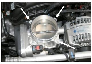
2. Remove the four bolts that secure the throttlebody to the intake manifold. Without disconnecting the wiring harness, remove the throttlebody from the intake manifold and set it
