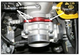
**4.** Install the Poweraid Spacer between the throttlebody and the intake manifold with the first supplied gasket next to the intake manifold, and the second supplied gasket next to the throttlebody as shown. Make sure the "flow" arrow printed on the spacer is pointing towards the intake manifold. Install the provided bolts and washers thru the throttlebody and the Power show and the Power show the throttlebody and
