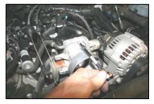
**3.** Using a 4mm socket, remove the three studs that hold the throttle body to the intake manifold. No need to remove the throttle body, leave it hang where it is.
