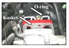
**6.** Place one fiber gasket (#4) between the Poweraid spacer (#1) and the throttle body. Make sure the flat face of the Poweraid spacer is against the throttle body with the bore extending into the intake manifold. **Use caution to retain the factory o-ring gasket on the intake manifold.**
