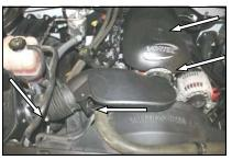
1. **Disconnect the negative battery cable!** Loosen one bolt and remove the beauty cover. Pry the tube from the clamp on the radiator hose. Loosen the hose clamps on each end of the intake tube and remove the tube.
