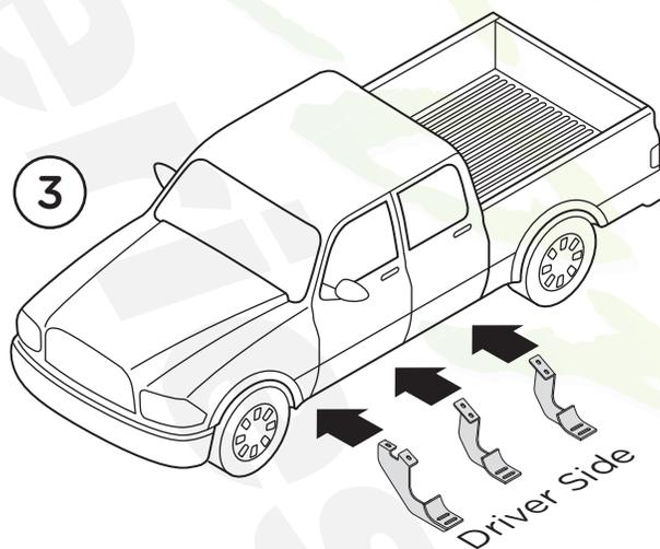
**4.** Align the Front, Center and Rear Driver's Side Brackets with the indicated holes located on the Rocker Panel of the vehicle.
