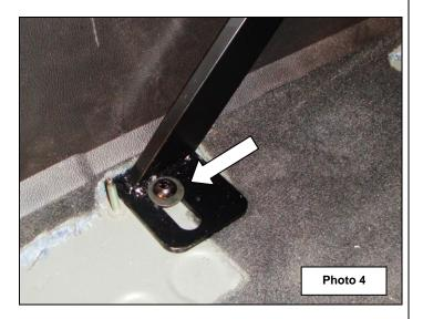
**Step-6** With assistance move the window assembly with the attached headliner filler panel into the vehicle. Position the window frame bottom rail on top of the main panel flange and align the (3) attachment holes in the window frame rail with the holes in the main panel. Attach the window frame rail to the main panel using (3) 1/4" x 3/4" button head screws and (3) 1/4" serrated hex nuts, (Photo 5). Leave the screws and nuts loose for final adjustment.
