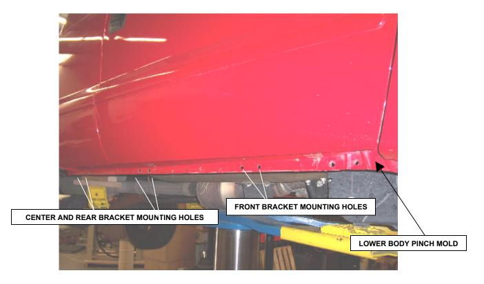
**Step 2.** This installation uses three mounting brackets per side. Beginning with the passenger side, locate the holes in the rocker panel and lower body pinch mold.
