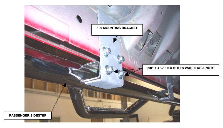
**Step 4.** Position the passenger sidestep up to the mounting brackets and loosely attach it to the brackets using the 3/8" x 1 1/4" hex bolts, washers and nuts as shown.
