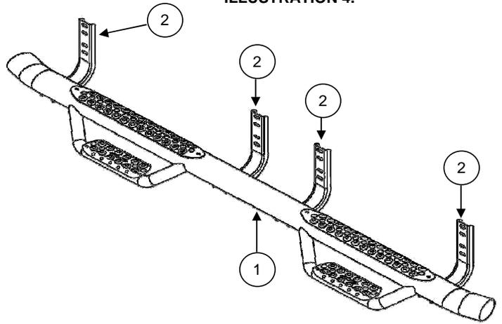
7.- Make any final adjustments to the alignment of the bracket and tighten all bolts.
