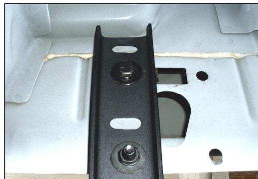
6.- Mount the side bar to the brackets and attach with: 5/16 x 1 1/4" hex head bolt, 3/8" flat washer, 5/16" lock washer. By each bracket. Leave loose. SEE ILLUSTRATION 3 & 4.
