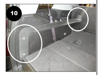
**Step-**9 With assistance, move the window assembly in to the vehicle through the rear cargo area. Position the base of the window frame on top of the partition main panel, and the window support brackets on the outside of the struts.
