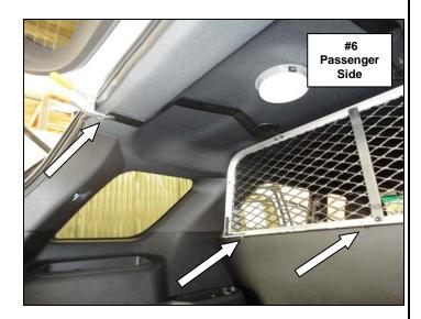
**Step-7** Pull the weather stripping away from the door opening. Hook the passenger side center bracket between the plastic molding and the vehicle pinch weld. Align the attachment hole in the center bracket with the hole in the main panel and secure the center bracket to the front of the main panel using (1) 3/8" x 3/4" button head bolt and (1) 3/8" serrated hex nut, **(Photo 7)**.
