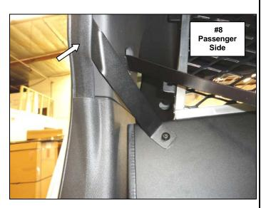
**Step- 10** With the upper brackets clamped in place, use the hole in the bracket as a guide and drill a 9/32" hole through the head liner and hatch opening, **(Photo 9)**. Secure each upper bracket using (1) 1/4" x 1 1/4" button head bolt, (1) 1/4" flat washer, (1) 1/4" rubber washer (place the rubber washer on the outside) and (1) 1/4" serrated hex nut.
