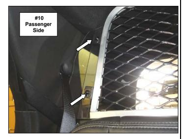
Step-12 Tighten all supplied and factory nuts and bolts as required and reinstall the front section of the plastic cargo area mat.
