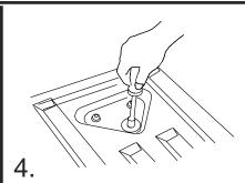
Place the 1/4-20 hex bolt with the appropriate washer into the rear and screw it into the POP&LOCK.
