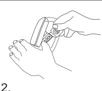
Lift the handle and insert the POP&LOCK between the handle and the plastic insert.
