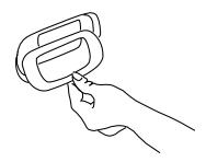
NOTE: POP&LOCK is designed to secure the passenger side latch. You may experience that the drive side latch can open due to the flex in the handle, but the tailgate will still remain locked.
