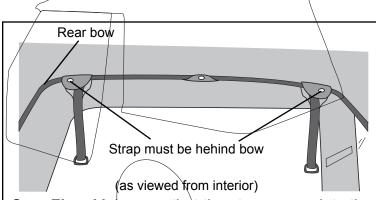
**Step Five:** Make sure that the straps sewn into the rear of the top are behind the rear bow.
