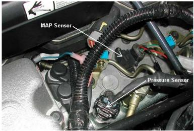
connector into the stock pressure sensor on the engine and the stock engine wiring harness connector into the supplied pressure sensor connector.
