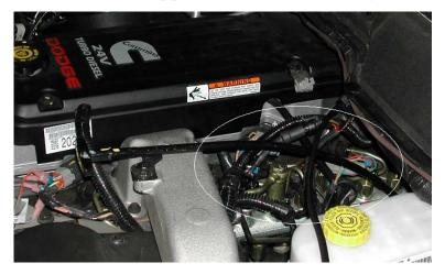
the engine compartment. Disconnect the stock wiring harness at the MAP sensor located on top of the intake manifold. Plug the supplied MAP sensor connector into the stock engine MAP sensor and the stock engine wiring harness connector into the supplied MAP sensor connector.
