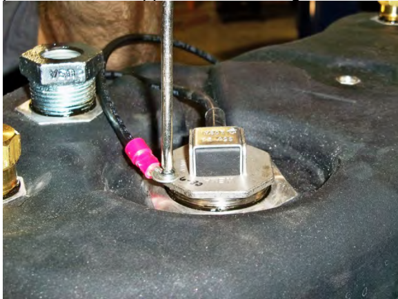
(Fig. 8) Connecting small eyelet end of grounding wire to top of electric fuel sensor. Other end to chassis frame.
