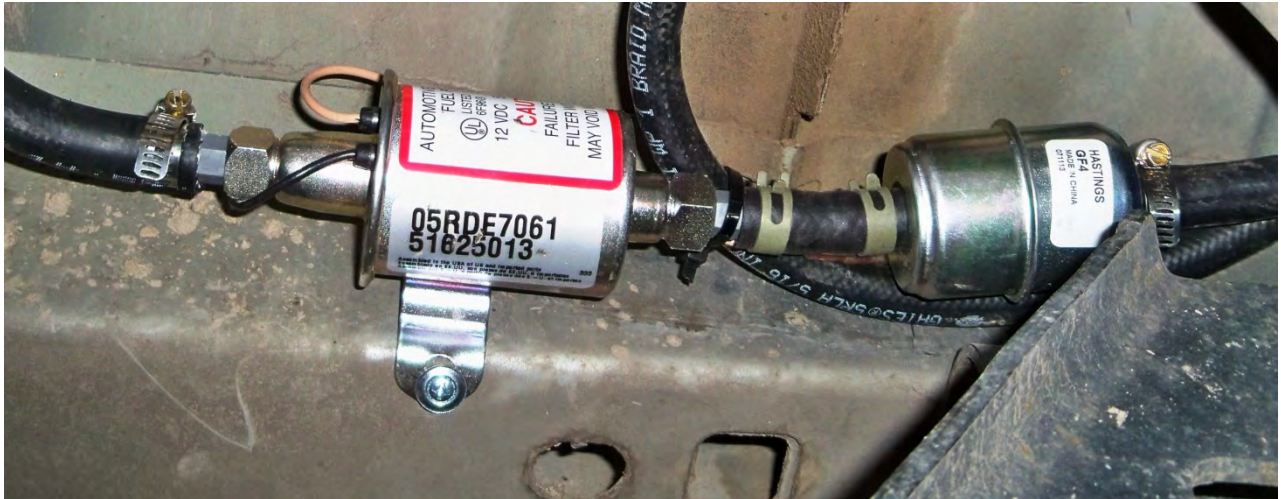
(Fig. 14) Fuel pump and inline filter installed.
