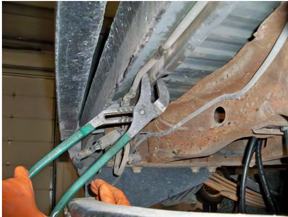
(Fig. 12) Using appropriate tools, bend or trim any sharp edges that come in contact with, or obstruct hoses.
