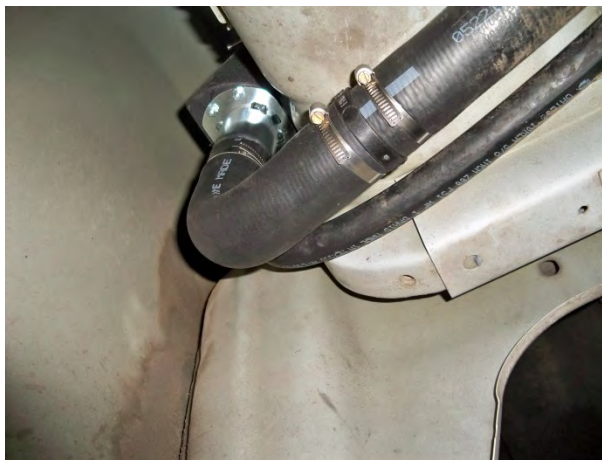
(Fig. 18) Check to be sure there is room in the fender space for the Poly Fuel Neck Flange Assembly BEFORE cutting any holes. Always test fit FIRST. Some fender spaces may require the trimming of sheet metal components to allow proper fit.
