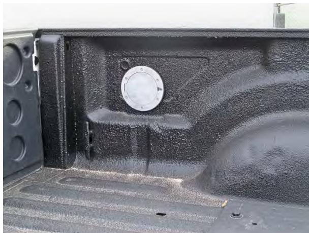
(Fig. 17) Location of Fuel Door located inside of bed wall.
