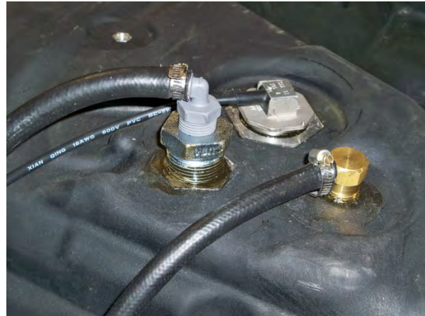
(Fig. 7) Install 5/16" hose onto the rollover valve
