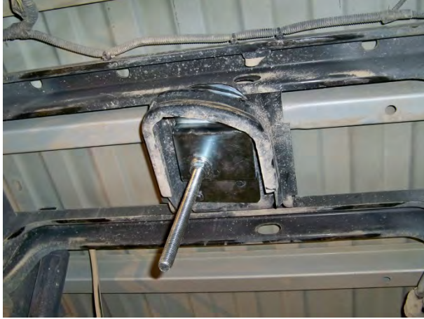
(Fig. 2) Cross member in 03-12 RAM vehicles showing STAFS top Truck Mounting Plate and Threaded Rod installed.
