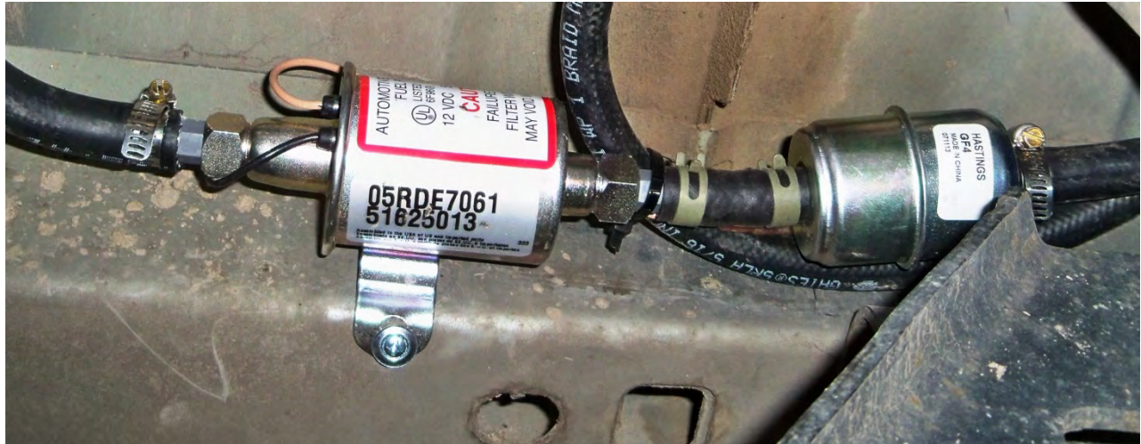
(Fig. 14) Fuel pump and inline filter installed.
