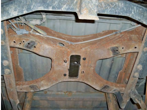
(Fig. 2) Cross member in 99-04 Ford vehicles showing STAFS top mounting plate installed.
