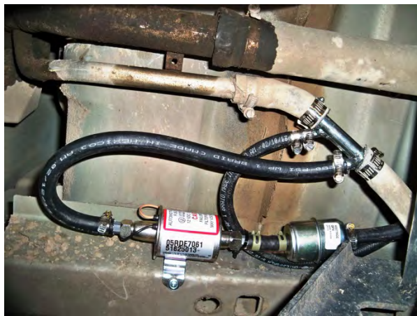
(Fig. 15) Vent Fill Neck Adapter installed.
