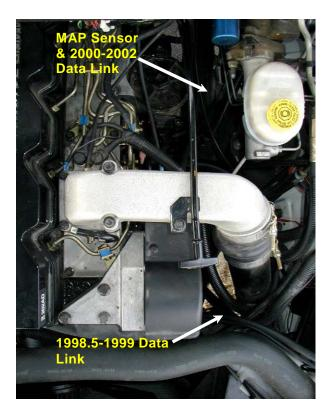
15.A plug is installed in the data link connector on the truck to resist corrosion, remove this and install the supplied connector.
