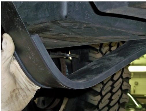
(Fig. 4) If optional TITAN Shield is not to be installed, install rubber bushings (pn 99 0000 0103) on both straps with the channel side toward the strap.
