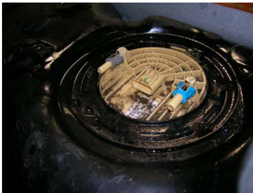
(Fig. 2) Loosen the hold-down ring on the OEM tank by turning counter-clockwise. Note where the connections on your vehicle’s sending unit are “clocked” and install so they are located in the same position in the new tank.
