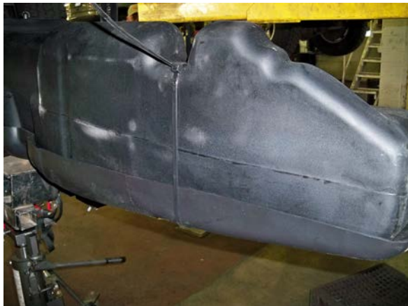
(Fig. 6) On 7030303 tanks only, if the optional Custom Shield is installed be sure to use the included Quick Tie to hold the shield securely to the front section of the tank as shown here. Trim any excess Quick Tie
