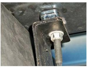
(Fig. 13) Thread two shims onto each strap bolt. (Fig. 14) Tighten the bolt and bracket against the shims. If the strap does not hold the tank tightly enough, remove one shim at a time until it is tight.
