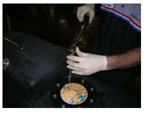
(Fig. 4) Tighten nylon locking nuts on the top flange to 20 ft. lbs of torque. Tighten in a "star" pattern.
