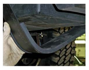
(Fig. 6) If TITAN™ Shield is NOT to be installed with the tank, then install Rubber Strap Bushings in tank mounting strap. Center the bushings in the bottom of the straps.
