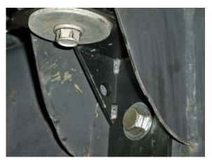
(Fig. 11) As an alternative to drilling the frame, the cab mount gussets can be drilled in-line with the "S" Bracket gussets and bolted into place. See the holes in the bracket gussets shown above.
