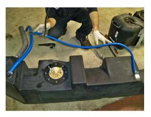
(Fig. 5) This shows final configuration for vent line system. Vent line on side of Vent Kit Assembly farthest from ¾" vent line should be left loose as it will not be connected permanently until tank is lifted into place and ½" vent line hose is threaded over the top of the truck frame. Vent system and fill hose is seen as follows (starting at the photo's right side and working counter-clockwise):
