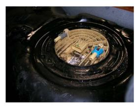
(Fig. 2) Be sure to clean the sending unit and surrounding area before removing sending unit.
