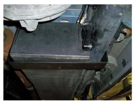
(Fig. 12) Photo shows the "S" Bracket Support installed at the front of the tank.
