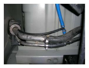
(Fig. 8) Photo shows final installation of fill hose and vent line hoses on vehicle's fill spout. Note the ¼" Vent Kit Assembly hose is securely fastened to the fill spout. The ¼" vent is necessary to prevent vacuum build-up in your TITAN™ fuel tank.
