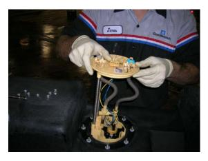
(Fig. 3) Carefully place sending unit into the TITAN™ fuel tank on top of "O" ring gasket.
