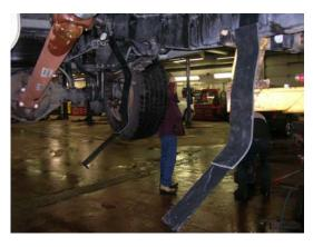
(Fig. 7) Carefully bend straps down out of the way in preparation for lifting tank into place.
