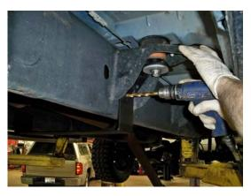
(Fig. 10) This shows the "S" Bracket Support bolted to the cab mount below the driver's door. As shown, drill a hole through the vertical center-hole of the bracket and fasten with the bolt provided.
