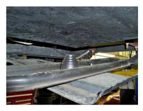
(Fig. 9) This photo shows the Cushion Mount installed on the factory skid plate below the tank.
