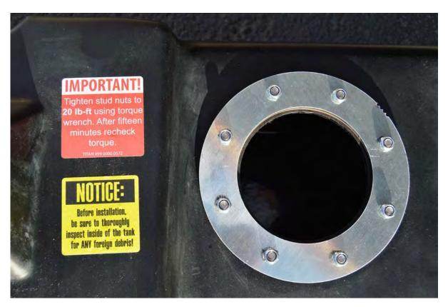
(Fig. 7) The sending unit top flange and installation notices are shown here.
