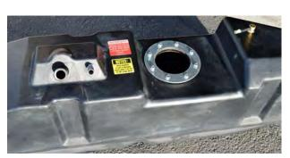
(Fig. 10) Install the OEM 1 ½" fuel tank fill hose to the large king nipple and the ¾" OEM vent hose to the smaller nipple. Be sure to fasten tightly with the OEM hose clamps.
