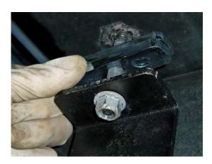
(Fig. 8) Thread two shims onto each strap bolt.
