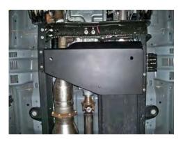
**Note:** Most late model Heavy Duty Ford truck models already have the frame drilled to accept the skid plate. If you come across a vehicle which does not, follow the placement instructions, clamp the skid plate into position and drill the bottom flanges of the frame to accept it. If your vehicle already has a factory skid plate, simply remove it and replace it with this one.
