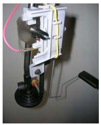
(Fig. 5) Level sensor in original forward facing position. Loosen the small hex head screw at the bottom of the sensor, carefully lift the sensor assembly off its mounting bracket. Rotate the sensor 180  $^{\rm o}$  and slide it carefully back onto its mounting bracket.
