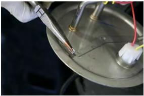
(Fig. 3) Leave the "O" ring gasket, studs and retainers assembled as they are (shown before sending unit, top flange, and 3/8" nylon locking nuts are installed).
