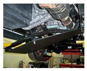
(Fig. 4) Attach the Skid Plate to the bottom of the passenger side of the frame first, leaving the bolts loose. Make sure the Nose Bracket is on the edge of the Skid Plate closest the rear of the vehicle.
