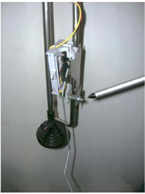
(Fig. 6) Level sensor has been removed and turned so as to face toward the rear of the truck when installed in the fuel tank. It is secured with pan-head screw, spacer (either steel or nylon) and nut. Pointer is indicating position of screw, nut and spacer.
