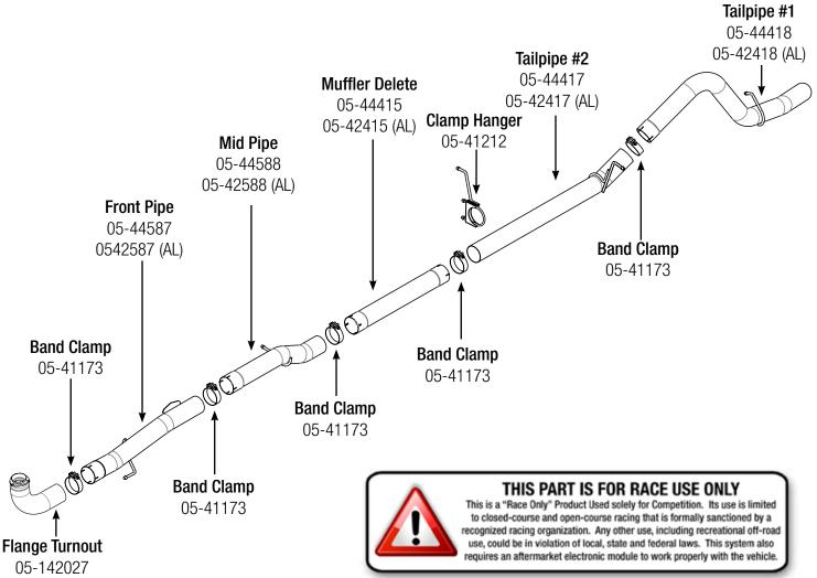
Step 1: (Read Instructions prior to installation) Remove the stock exhaust from the rear of the truck working your way forward. Take caution not to damage the factory isolation mounts as they will be reused. Disconnect sensors at the connections. Take caution as not to damage any sensors. It is recommended to not fully tighten the clamps until the entire system has been installed.
