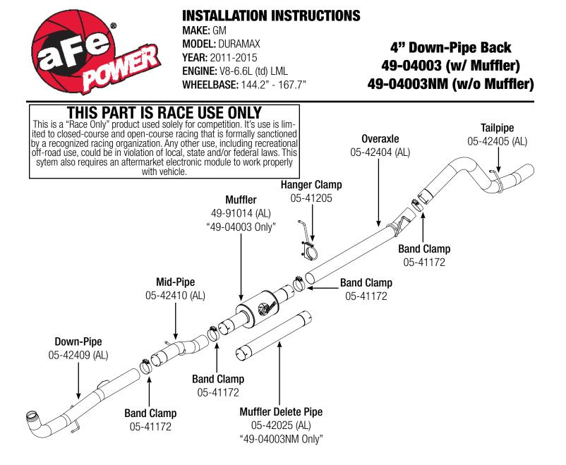
Step 1: (Read Instructions prior to installation) Remove the stock exhaust from the rear of the truck working your way forward. Take caution not to damage the factory isiolation mounts as they will be reused. Disconnect sensors at the connections. Take caution as not to damage any sensors. It is recommended to not fully tighten the clamps until the entire system has been installed.
