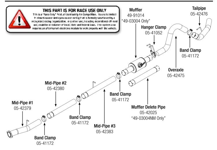
**Step 1: (Read Instructions prior to installation)** Remove the stock exhaust from the rear of the truck working your way forward. Take caution not to damage the factory isiolation mounts as they will be reused. Disconnect sensors at the connections. Take caution as not to damage any sensors. It is recommended to not fully tighten the clamps until the entire system has been installed.
