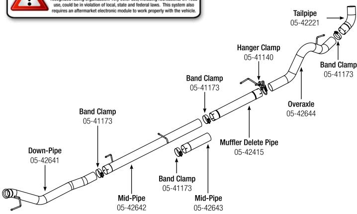
Step 1: (Read Instructions prior to installation) Remove the stock exhaust from the rear of the truck working your way forward. Take caution not to damage the factory isiolation mounts as they will be reused. Disconnect all sensors and urea injector at the connections. Take caution as not to damage any sensors. It is recommended to not fully tighten the clamps until the entire system has been installed.
