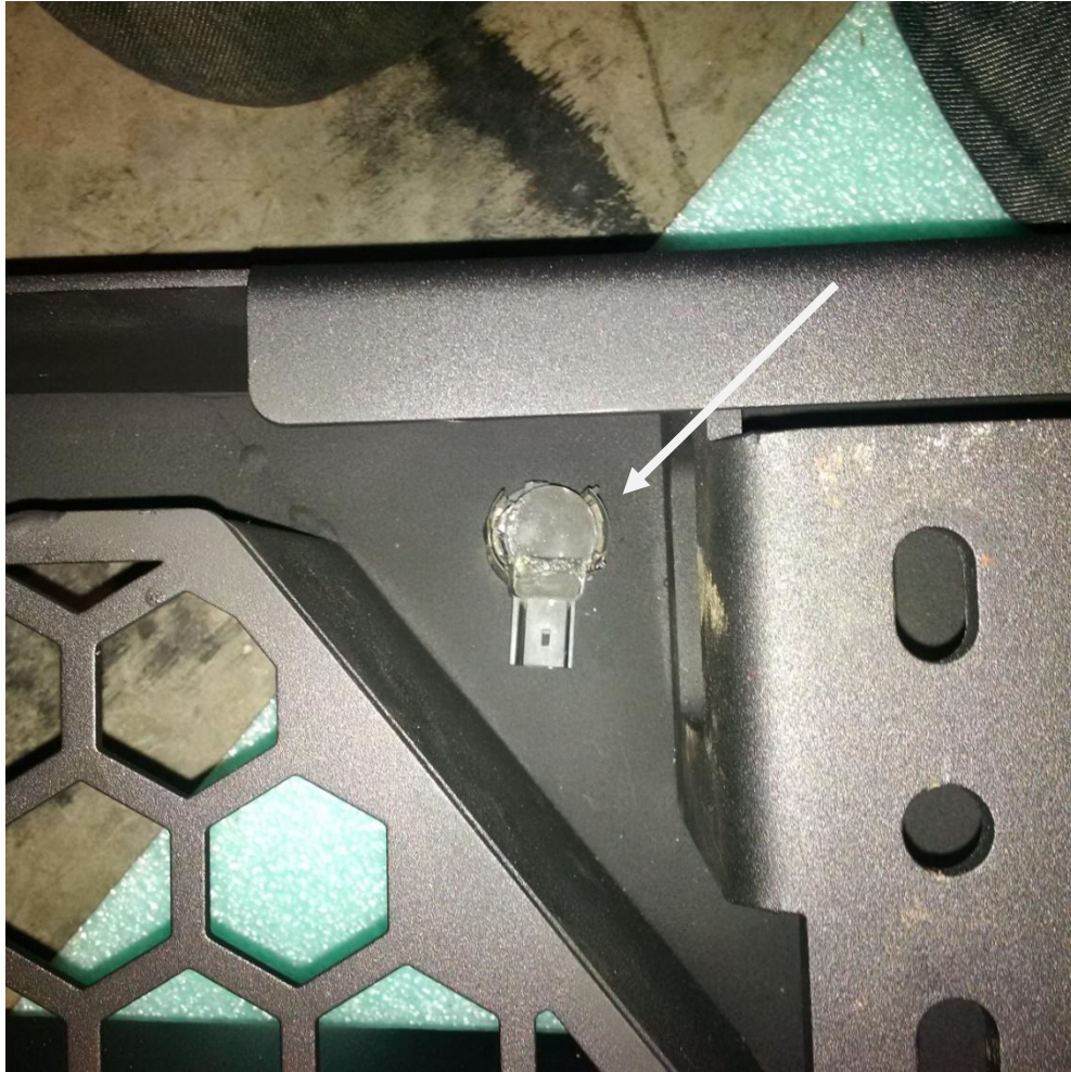
Figure 4 Outer passenger side sensor orientation
