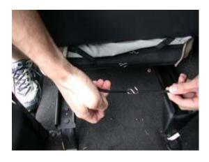
(ATTACH 2 ENDS OF THE TENSION CORDS TOGETHER AT BACK OF CUSHION)
