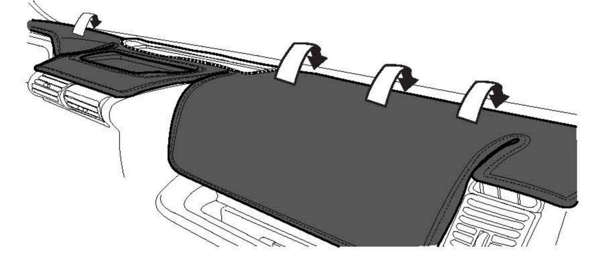
**TIP:** Because of auto assembly tolerances or variations in the position of replacement windshields, dash covers may require trimming on the windshield edge.
