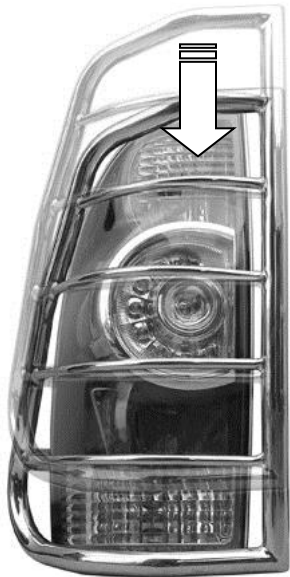
(Fig 3) Slide the Taillight Guard over the taillight assembly from the top down
