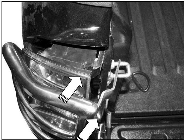
(Fig 5) Use both hands (one on bottom, one on top) to hold the Taillight Guard in place over the taillight. Slide the taillight and Guard into the opening in the rear fender
