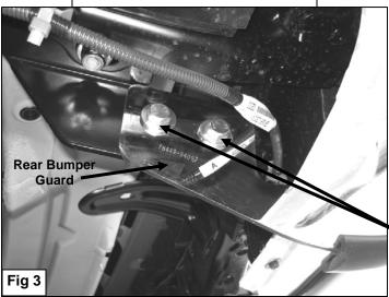
12mm x30mm Hex Head Bolts 12mm Lock Washers 12mm Hex Nuts 12mm Flat Washers
