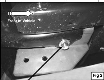
12mm x30mm Hex Head Bolt 12mm Lock Washer 12mm Hex Nut 12mm Flat Washer
