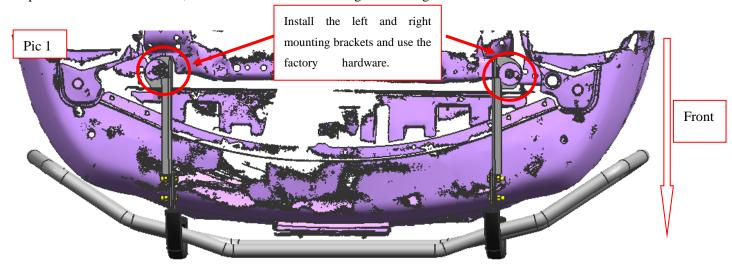
Step3: Refer to the pic 2 to install the front guard on the brackets, and then adjust the brackets.
