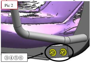
Step4: Check if all hard ware are installed and tighten up.
